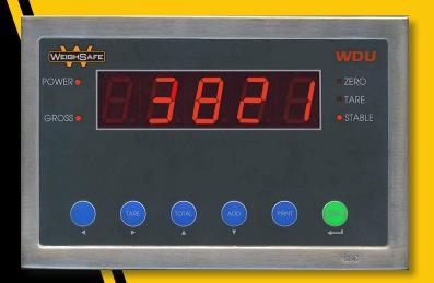
The **WEIGHSAFE WDU 2001** incorporates a micro-processor based unit connected to the hydraulic lifting system found on lift trucks or similar machines. A load is placed on the forks and is then accurately weighed by measuring the hydraulic pressure required to raise the load. The hydraulic sensor measures pressure and converts it to an electronic signal which is displayed on the WDU monitor.
