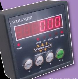
The WEIGHSAFE WDU MINI SERIES is a compact micro-processor based unit connected to the hydraulic lifting system found on lift trucks or similar machines. A load is placed on the forks and is then accurately weighed by measuring the hydraulic pressure required to raise the load. The hydraulic sensor measures pressure and converts it to an electronic signal which is displayed on the WDU MINI Monitor.
